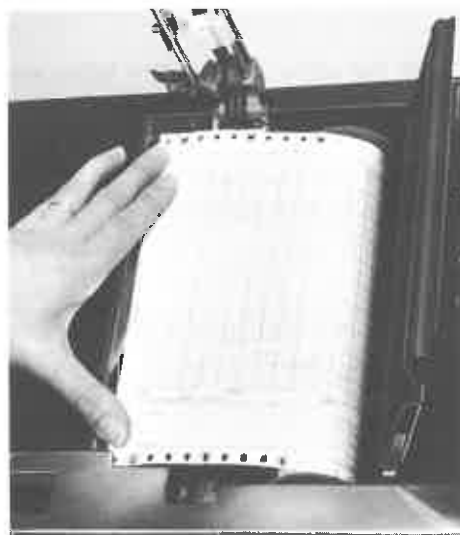
Fig. 2-5 Marked Sprocket and Perforation.
