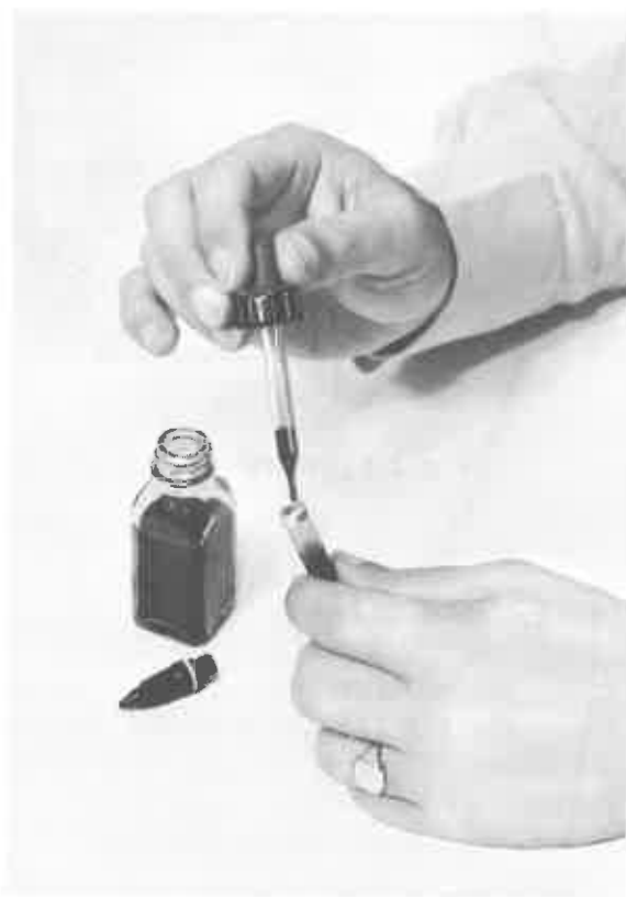
Fig. 2.3 Filling the Pen Reservoir
